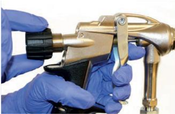
Figure 6.1: Connecting the braided hose to the container valve.
