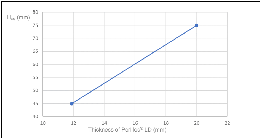
Figure A.2.4: Equivalent thickness of concrete (90 minutes).
