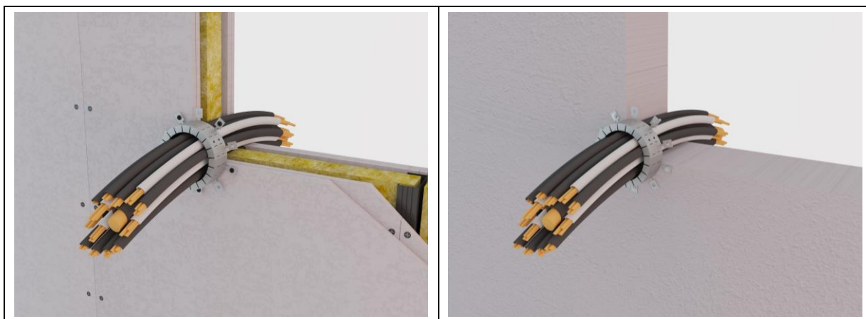
Figure B.6.1: Example of small sheathed cables penetration seal in a flexible or rigid wall.
